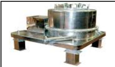
In basket centrifuges, the solids & liquids are separated by centrifugal force using a filter media (usually a cloth) mounted over the rotating basket
